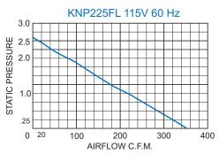
Airflow vs. static pressure curve is shown for 60 Hz (solid line) inputs. Static pressure is in inches of water.
